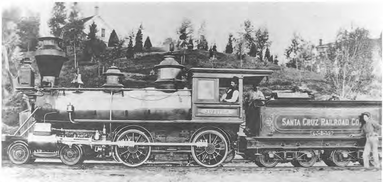
The Jupiter, a 4-4-0 wood burner similar to the ones that operated on the narrow gauge tracks from Santa Cruz, that met the flume from Waterman Gap at the town of Felton, circa 1875. Photo: Covello and Covello Historical Collection
